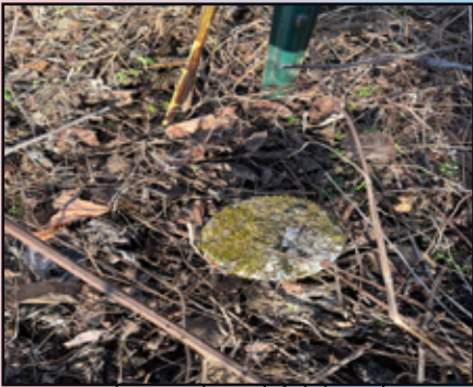
A marker hidden by debris and moss.
